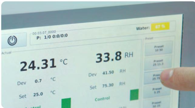
Due to the touch display, the measuring values are comfortable to control. The clear menu structure enables an intuitive and simple handling. Help texts are additionally at your disposal. With the touch display, the Huminator II can be programmed in a few steps. If required, this process can also be conducted via the USB interface.
