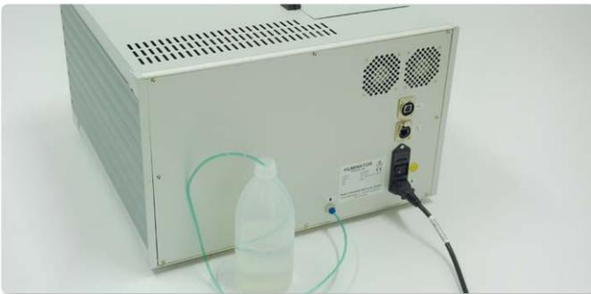
Illustration 8: Rear side of the Huminator II with connected hose to fill the system).
