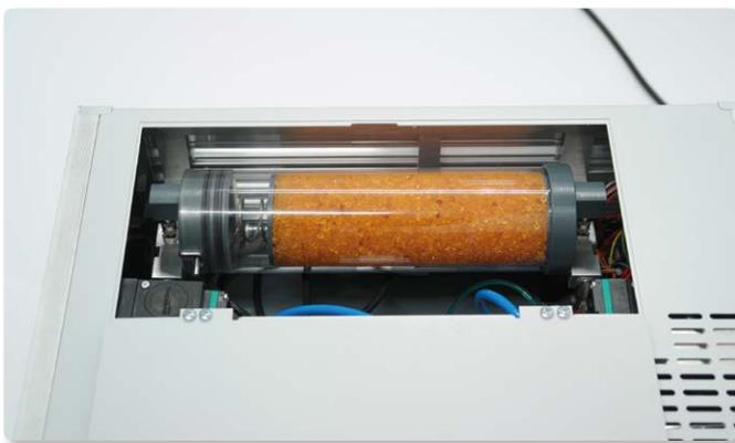
Illustration 5: Desiccant cartridge inserted in the Huminator II
