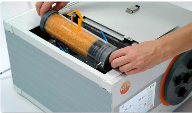
Illustration 28: Removing the desiccant cartridge
