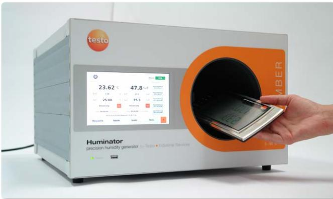
Illustration 15: Opened measurement chamber with weather station
